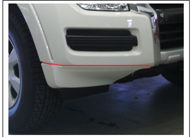
Figure 8: Cut line from flare to inner corner of plastic bumper cover.
